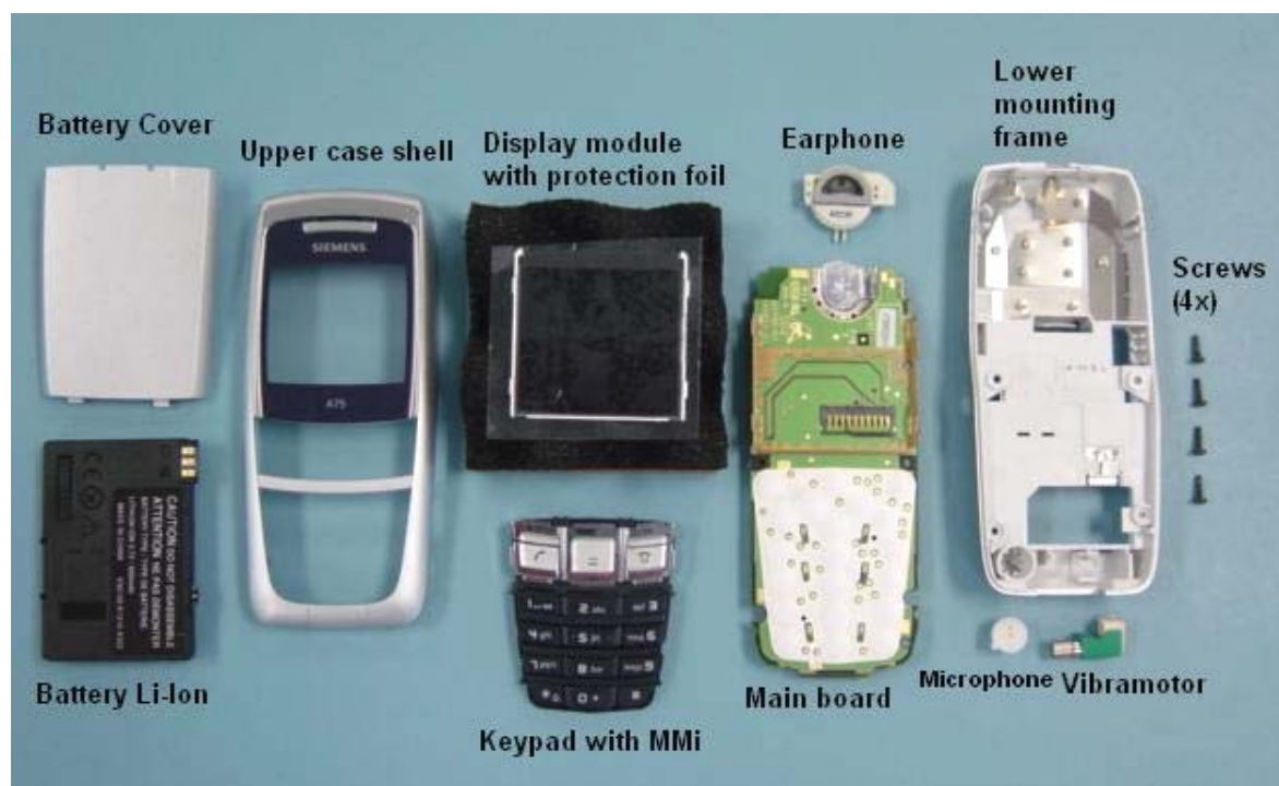
Fully disassembled A75
