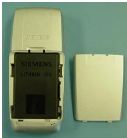
Remove Battery cover.
