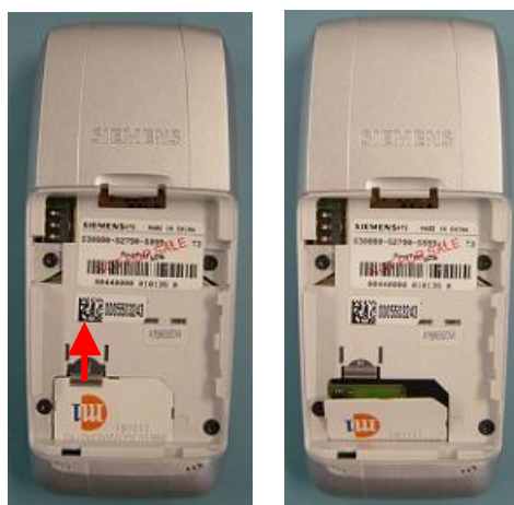
Remove SIM Card: 1) move latch upwards; 2) SIM Card will eject from holder
